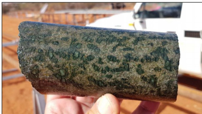
Coarse grained olivine in supergene sulphide groundmass - “leopard texture” (RKDD018, 114.2m HQ core)
