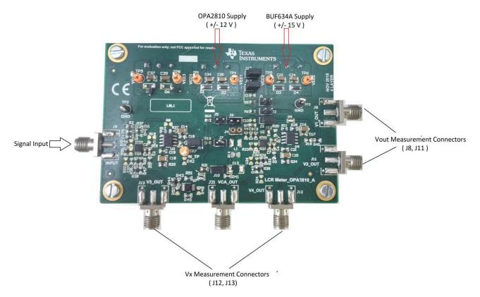
Figure 3-2. Board Connections
