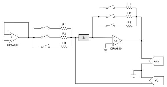
Figure 2-6. Impedance Measurement Design
