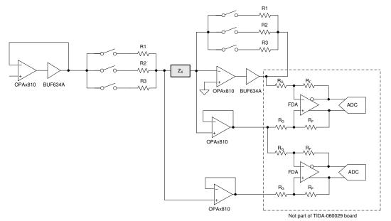
Figure 2-1. TIDA-060029 Block Diagram
