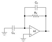
Figure 2-5. Capacitor Measurement Circuit w/ Compensation Capacitor
