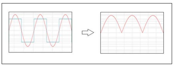
Figure 2-10. Square Wave Modulation
