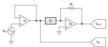
Figure 2-2. Basic Impedance Measurement Circuit
