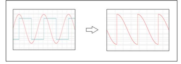
Figure 2-11. Square Wave Modulation with 90° phase
