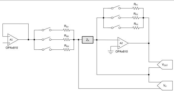
Figure 2-9. Method 1 of Impedance Measurement
