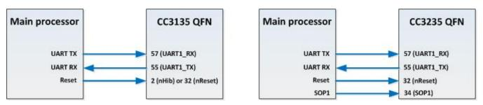
Figure 1. CC313x and CC323x QFN Programming Setup
