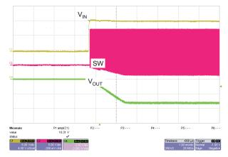
Figure 5. SW Node Voltage During Start-Up
