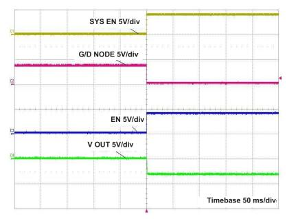
Figure 13. EN Pin Level Shifter on Start-Up
