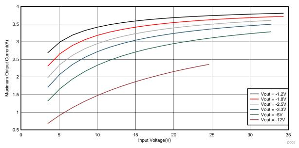
Figure 3. Recommended Maximum Output Current for LMZM33604
