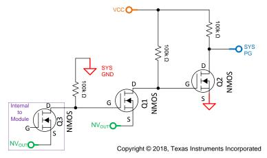
Figure 15. PG Pin Level Shifter
