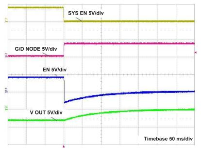
Figure 14. EN Pin Level Shifter on Shutdown
