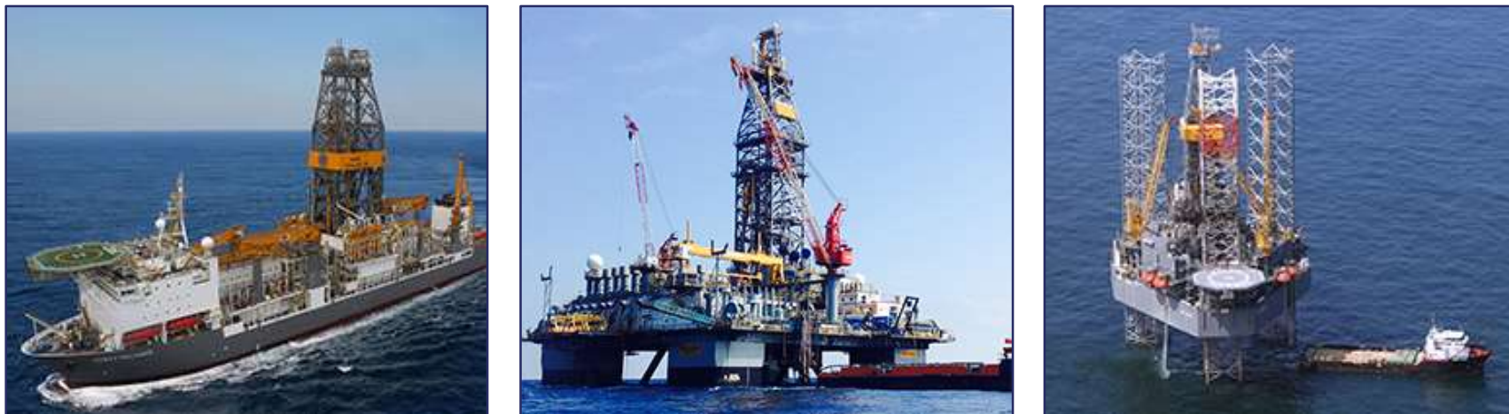
Figure 6: Various Offshore Drilling Rigs – From Left to Right a Drillship, Semi-Submersible, and Jack-Up Rig
