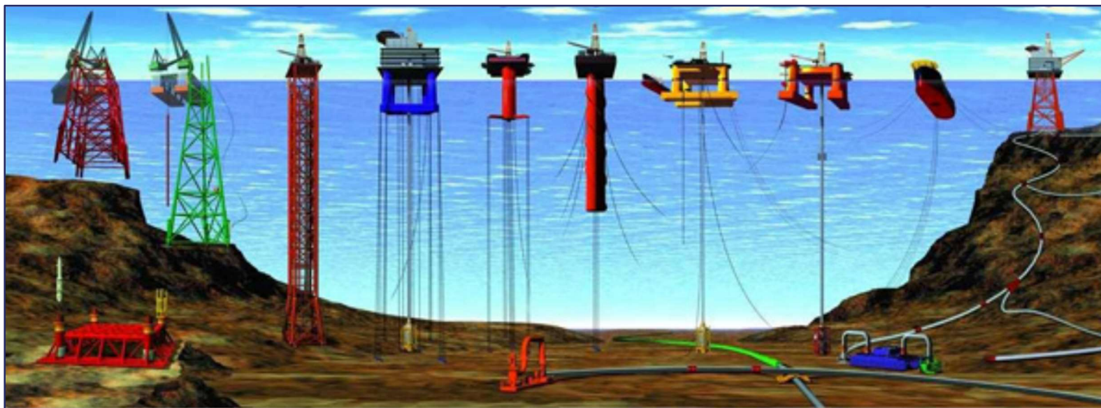
Figure 7: Types of Offshore Oil and Gas Facilities
