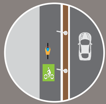
Protected Bike Lane
