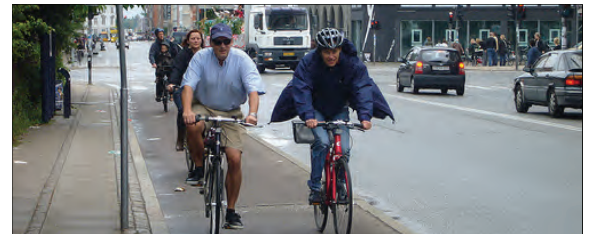
Figure 5-69. Protected cycle track
