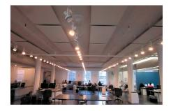
Dozens of bright point sources are used to provide general illumination to make room for acoustic panels
