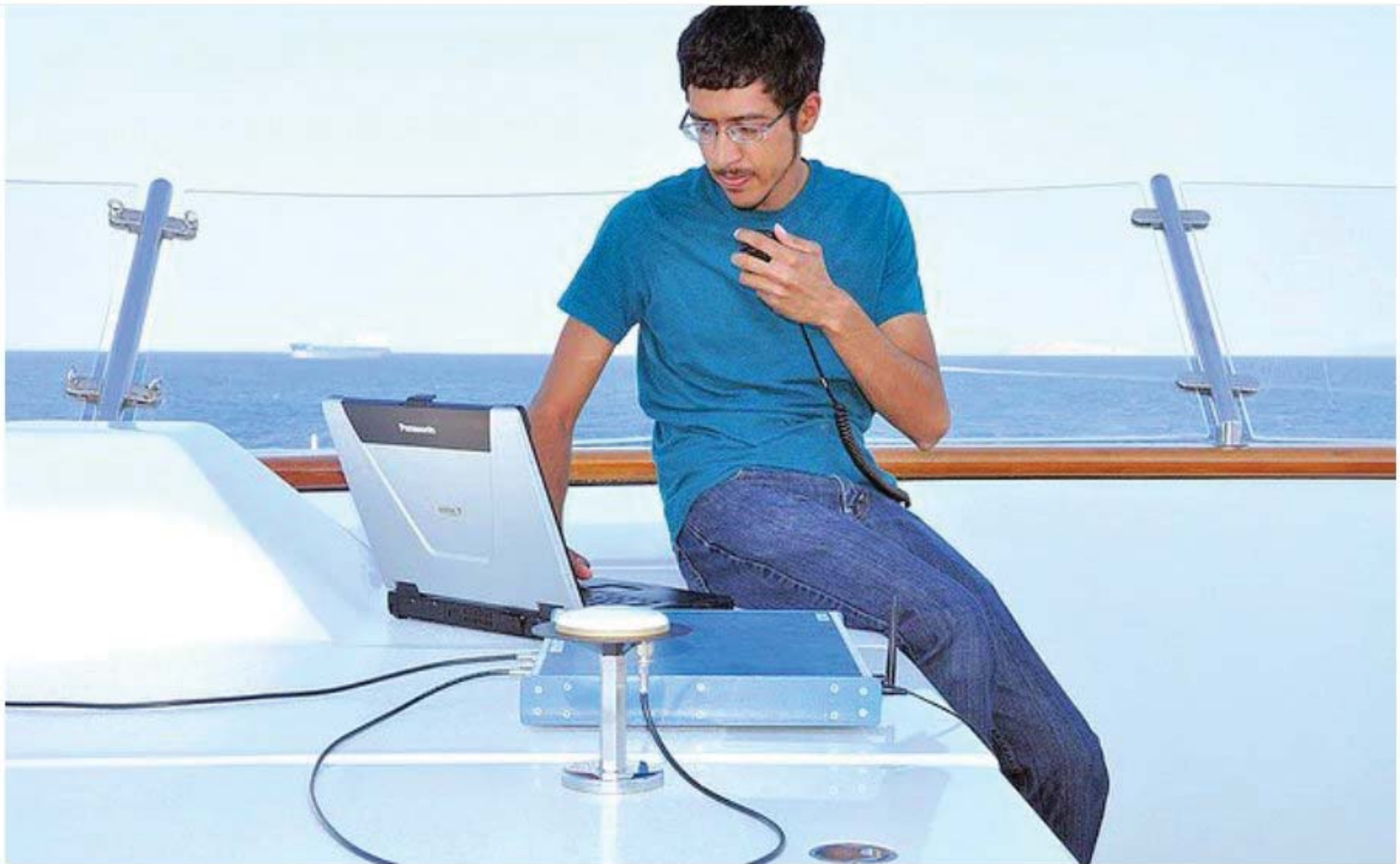
Jahshan Bhatti operates the spoofing hardware aboard the White Rose (Photo: UTexas at Austin)
