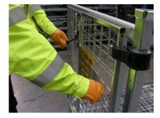
Lift out the top folding section of the folding gate, hinge outwards and fold down over lower half of gate.
