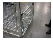
Using both hands slide the lower gate release catches inwards to release them from the outer posts. Lower the folded gate assembly into the FSC.
