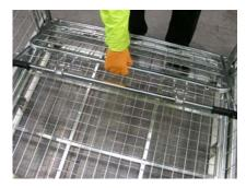
Lift the top folding section up and hinge down to sit flat against the FSC base. Step in if required.
