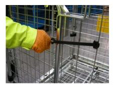
Hinge open LH full gate, secure against side panel with bungee strap.
